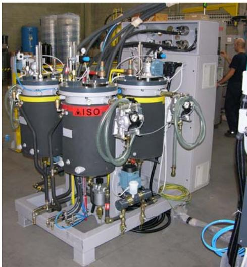
**Figure 16.** Cannon Gasketing Three Component Dosing Unit
