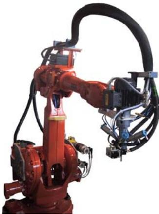
**Figure 18.** Cannon B1 Multi on ABB Anthropomorphic Robot
