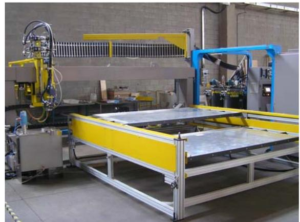
**Figure 14.** Standard Gasketing Plant with Cartesian Robot and Shuttle Table
