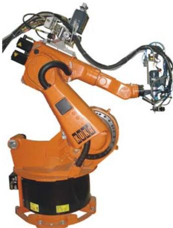
**Figure 19.** Cannon B1 Multi on KUKA Anthropomorphic Robot
