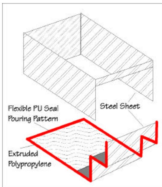
Picture 3: layout of a standard refrigerator cabinet in bent metal sheet, with the rear wall made with an extruded Polypropylene sheet
