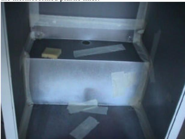
Picture 1: The conventional sealing of a refrigerator cabinet, before the introduction of the rigid Polyurethane foam, is usually made with adhesive paper-tape.
