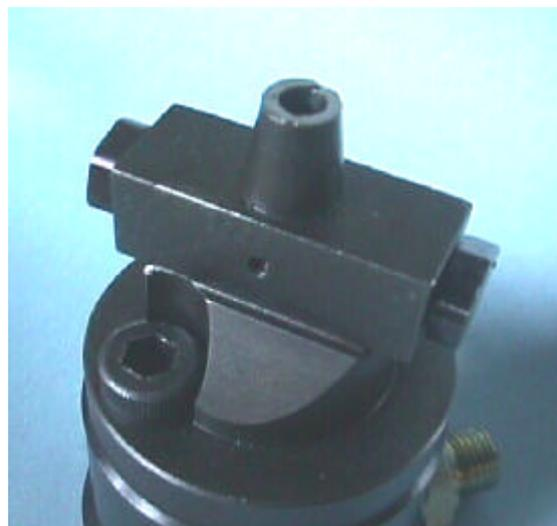
Picture 4: The Cannon LN5 mixing head used for this low-output medium-pressure injection
