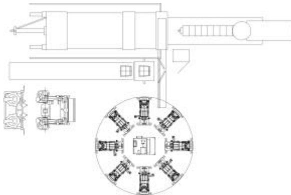
Picture 8: turn-table solution for the foaming side
