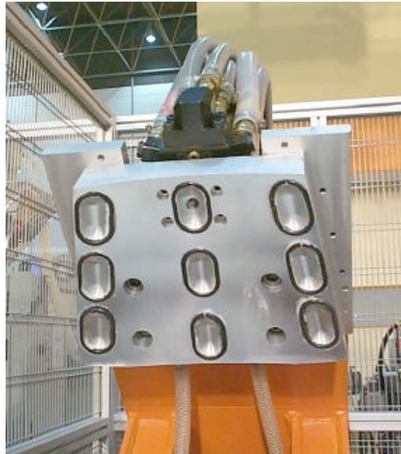
Picture 3: Details of the PUR-foaming mould
