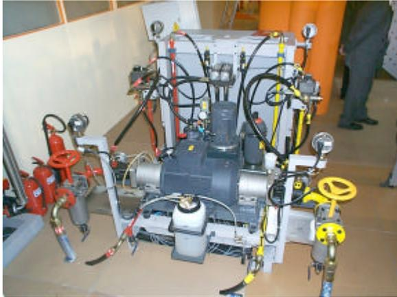
Picture 7: the Cannon "A-System 40" high-pressure metering unit
