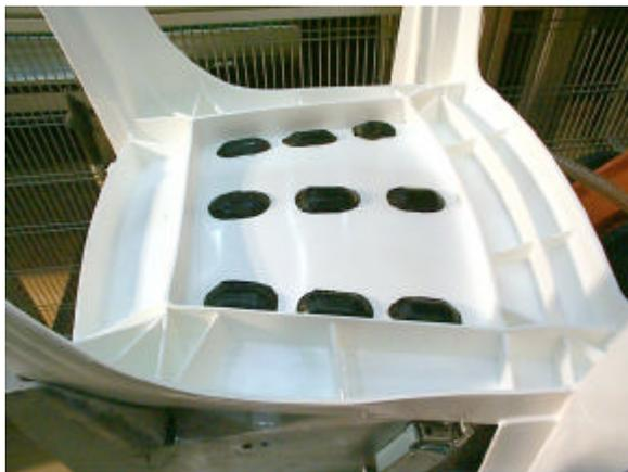
Picture 4: the 9 PUR buttons that hold the seat in place
