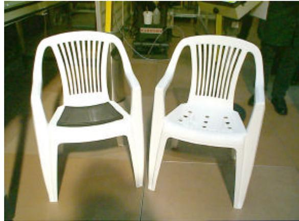
Picture 9: The finished garden chair (left) with a PUR integral skin foamed seat
