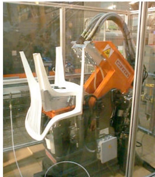
Picture 5: the foaming press, with a ready chair
