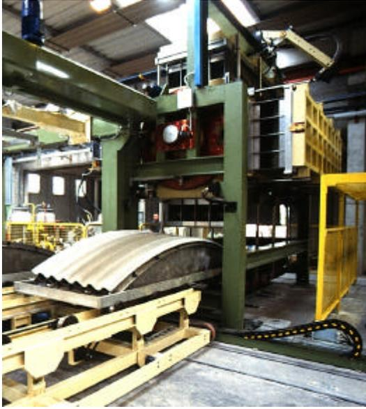
*Figure 8 – The use of Cannon proprietary Drum Unit - in a special version for curved roof panels – allows for the injection of four panels in the same foaming fixture, saving space and simplifying maintenance.*
