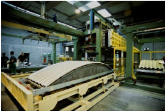
Figure 2 – A compact, highly-automated, dedicated solution has been designed by Cannon to produce insulated roof panels.
