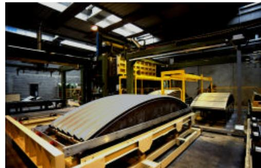
Figure 7 – Loading/unloading cart, servicing the assembly station
