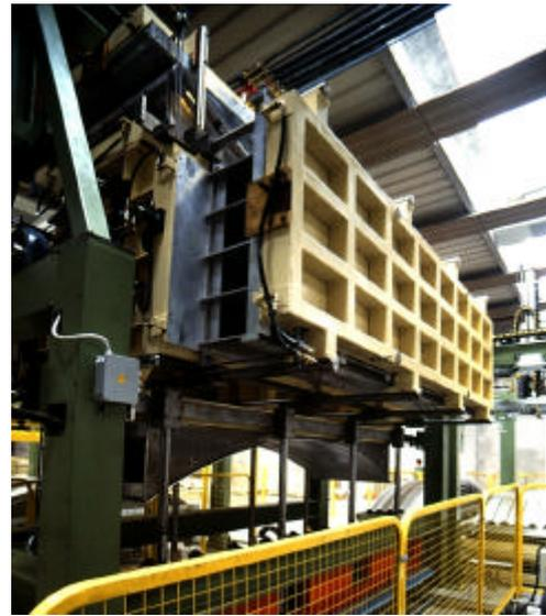
*Figure 9 – Loading and unloading are made using the lowest mould, while foam injection is performed in the uppermost.*
