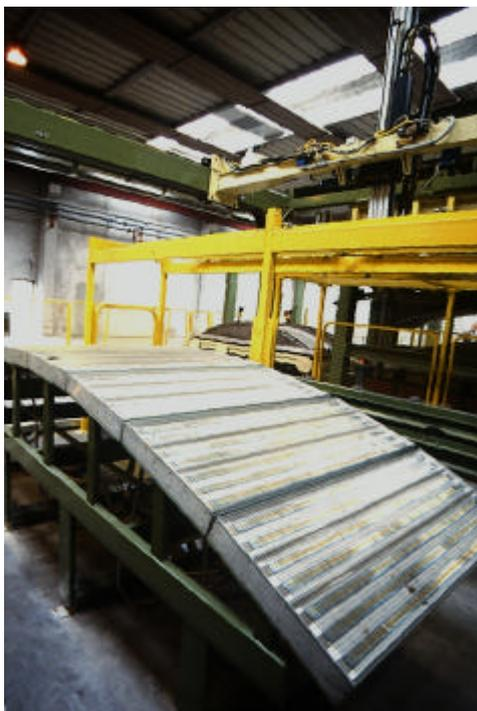
Figure 6 – Preheating station, with low-inertia Cannon MVL infrared elements
