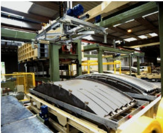
Figure 10 – Finished panels are automatically stacked in pallets after demoulding
