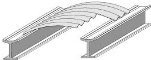
*Figure 1 – Old curved panels for roofs – often containing Asbestos fibers – can be replaced with new Polyurethane-insulated ones.*
