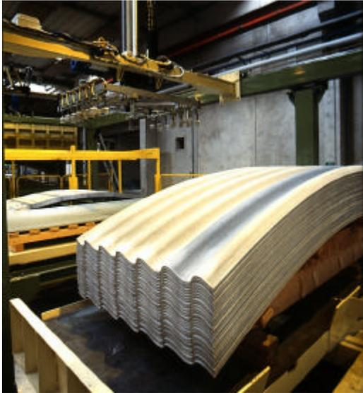
Figure 5 – The unloading/centring station for the upper facings
