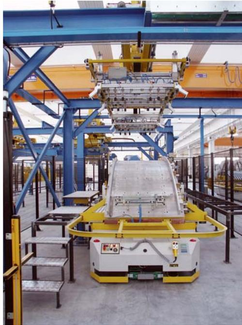
FIGURE 5: Automated Guided Vehicle (AGV)
