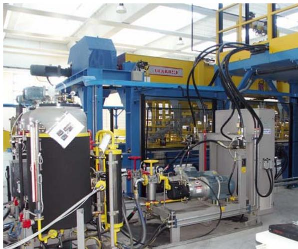
FIGURE 7: High Pressure Metering Unit
