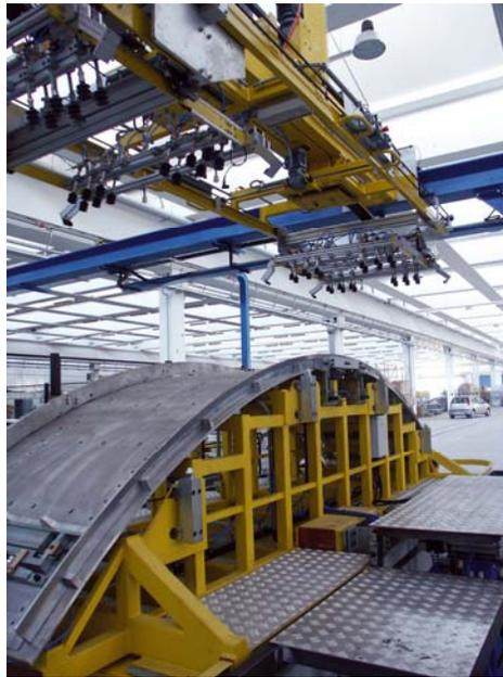
FIGURE 6: Outer Metal Liners Loading Station
