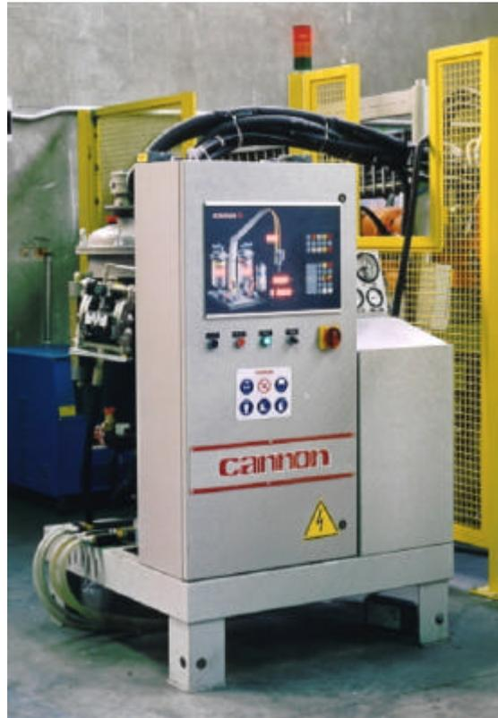
Picture 2: Cannon b2G, the dedicated machine and head developed for low-output, low-pressure dispensing of formulations for gasketing
