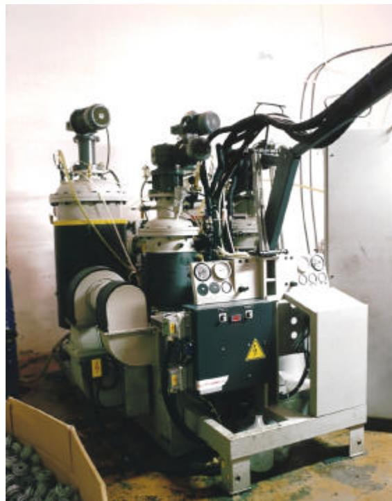
Picture 5: The special version of dispensing machine used for low-output applications with cast elastomers (skateboard wheels)
