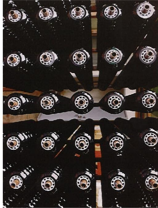
*Picture 8: Skate wheels ready for packing, after a short post-curing session at room temperature*
