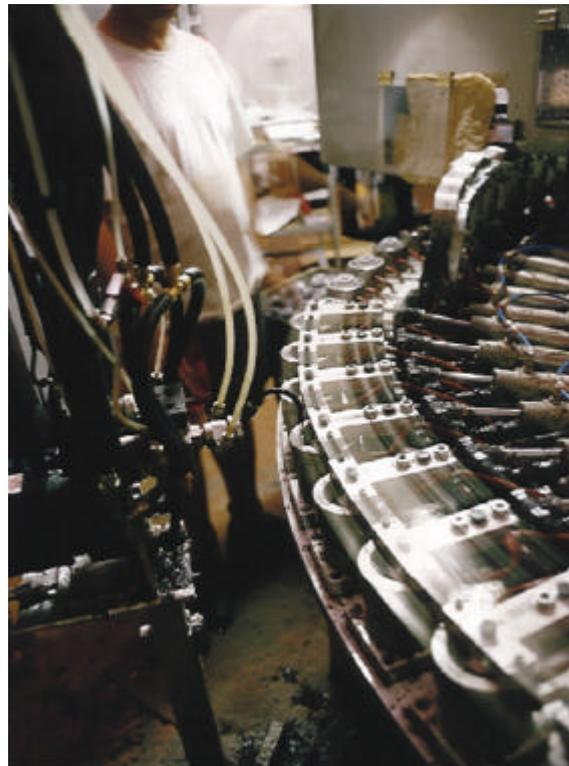
Picture 7: Turning tables with pneumatically-operated moulds are used for the production of these small items
