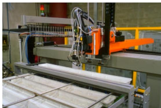
Picture 3: Cannon's pouring robot for gasketing
