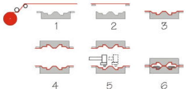
Figure 1. Cannon’s “Foam & Film” technology allows the polyurethane process to be fully automated by eliminating the need to clean molds or spray mold release.
