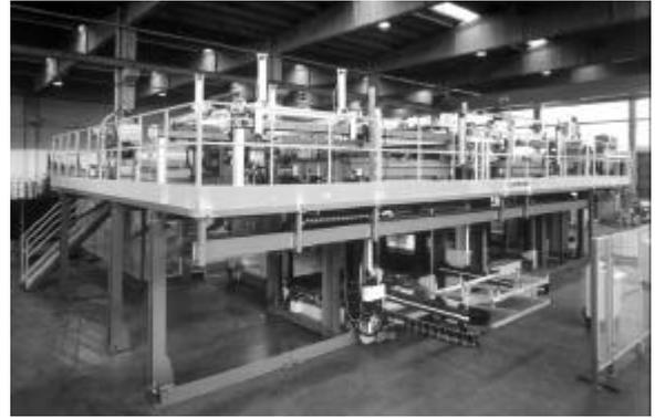
Figure 7. Cannon's continuous molding process for the production of industrial vehicle carpets INSOTEC incorporates "Foam & Film" technology to make manual intervention unnecessary.
