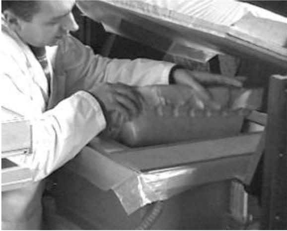
Figure 6. Parts made with releasing "Foam & Film" technology are removed from the mold while the film remains in the mold.
