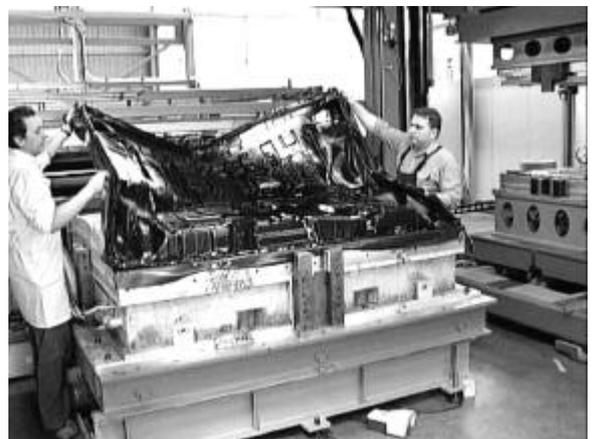
Figure 8. Sound-deadening vehicle flooring consists of a top "heavy layer", an intermediate sound-deadening polyurethane foam layer and a lower protective layer.
