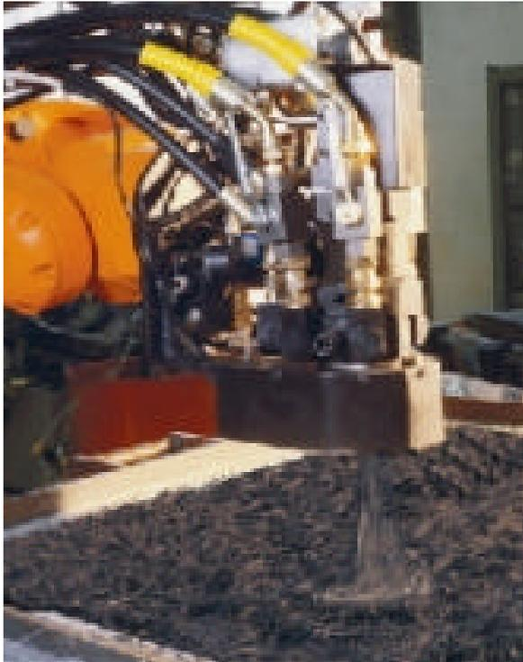
*Picture 4 - The pneumatic device provides very high-quality laydown of the blend*
