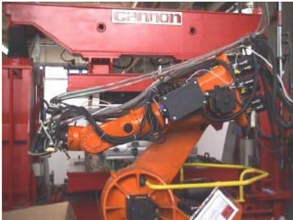
Picture 2 - Feeding the reinforcements from the storage to the mixing head requires a careful design of all the moving parts involved, to avoid any blockage.
