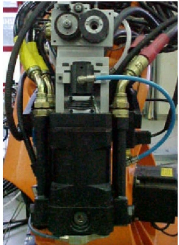
Picture 3 - The new InterWet head features a wider glass-chopper with higher output and longer life
