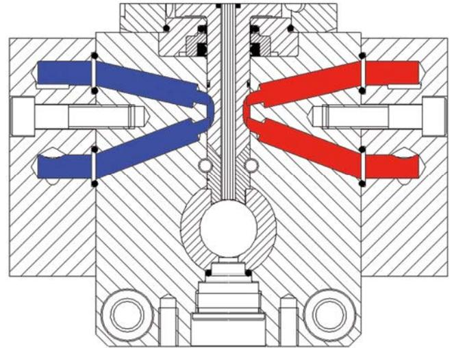
FIGURE 3: Discharge Piston Open
