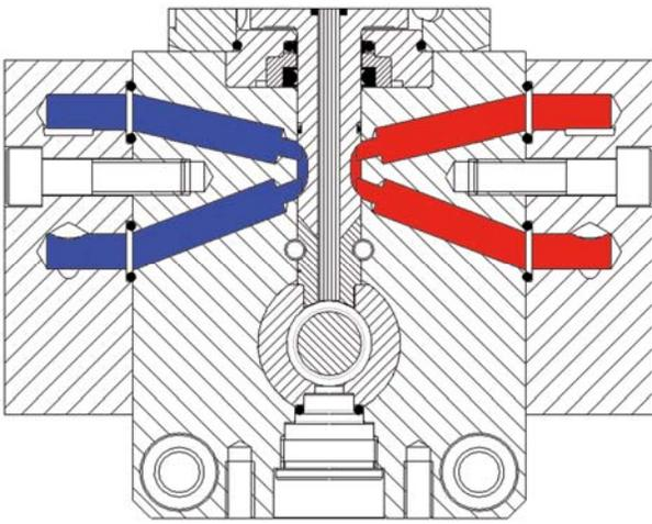
FIGURE 2: High Pressure Recirculation Through Mixhead
