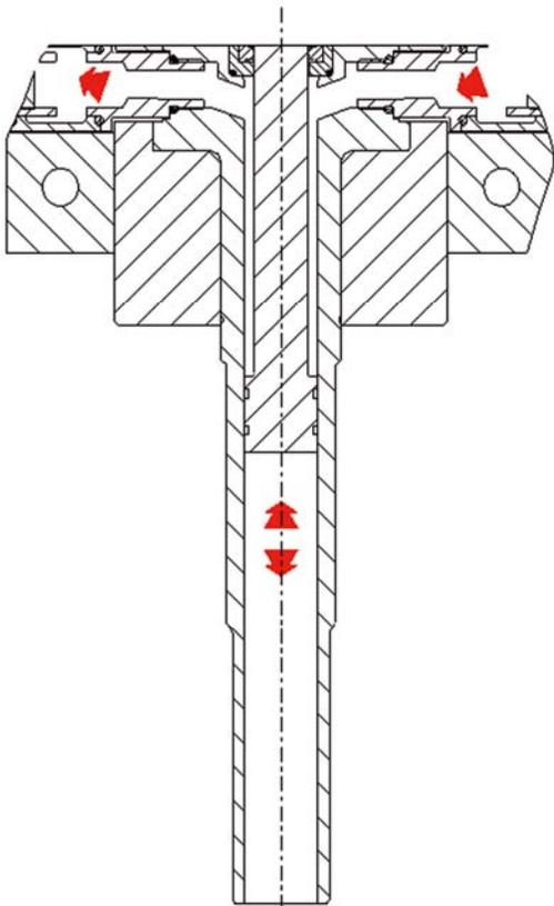
FIGURE 6: Mixhead Lubrication
