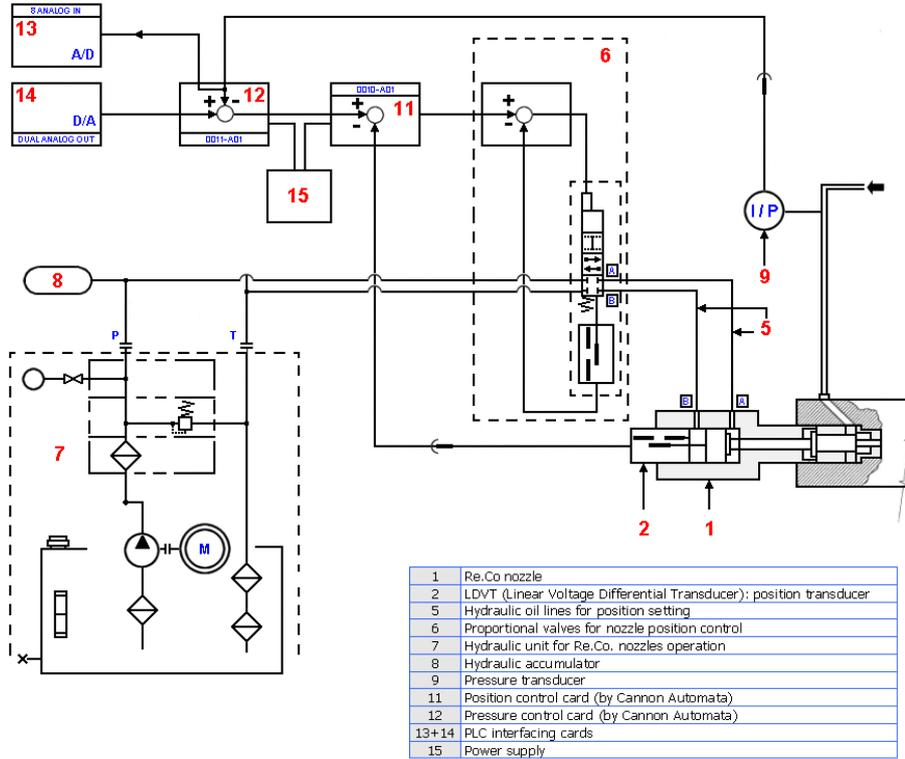
Picture 4 – Re.Co. Component Circuit
