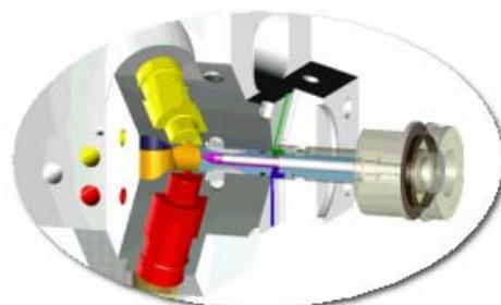
Picture 2: Pouring with radial and axial injection
