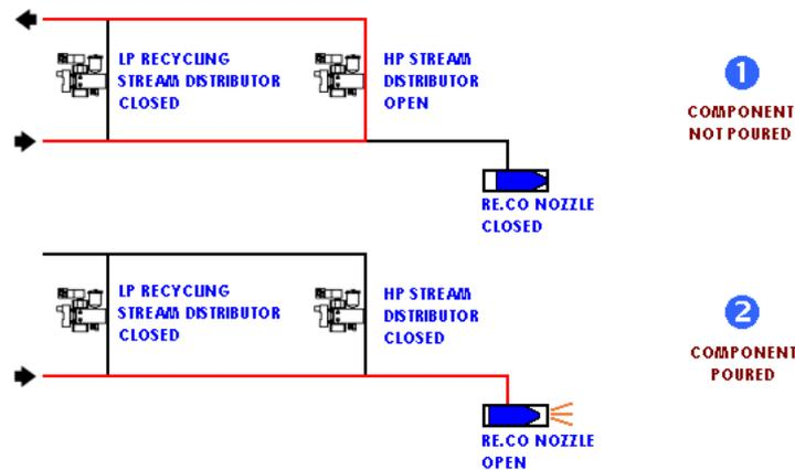
Picture 5 – Detailed view of the Re.Co. System: recycling/pouring phases through LP/HP by-pass stream distributors
