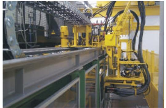
*Picture 4 - The 3-axes mixhead manipulators*
