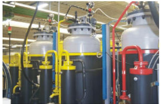
*Picture 6 - High pressure metering machines, with two different polyols availability*
