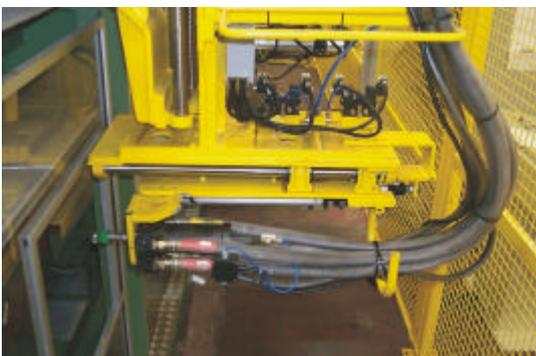
*Picture 7 - FPL self-cleaning mixing heads*
