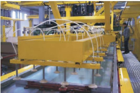
*Picture 5 - Pneumatic panel handling devices*
