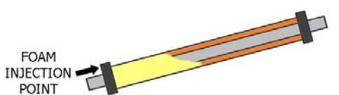
Picture 1 - Bottom-Up Filling Configuration
