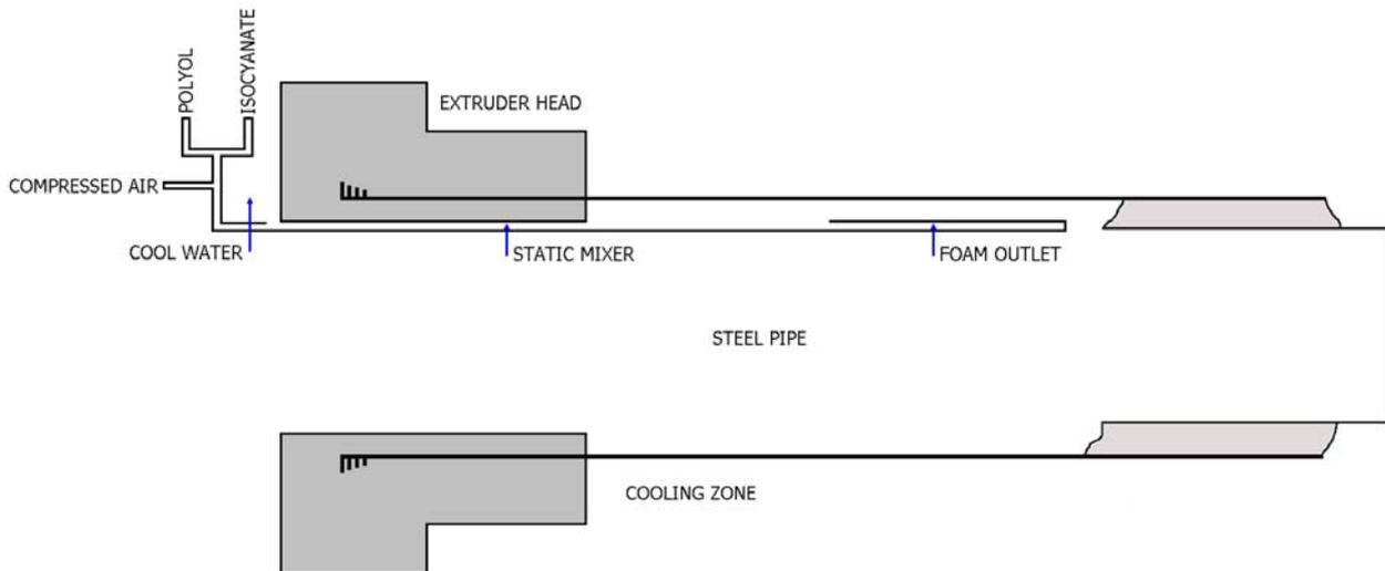
Picture 5 – Polyethylene Extruder and PU Foaming Layout
