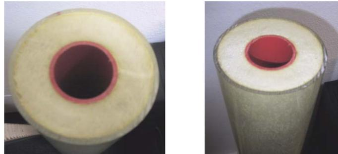
Picture 8 – Insulated Pipe-in-Pipe foamed during Lab's Trials
