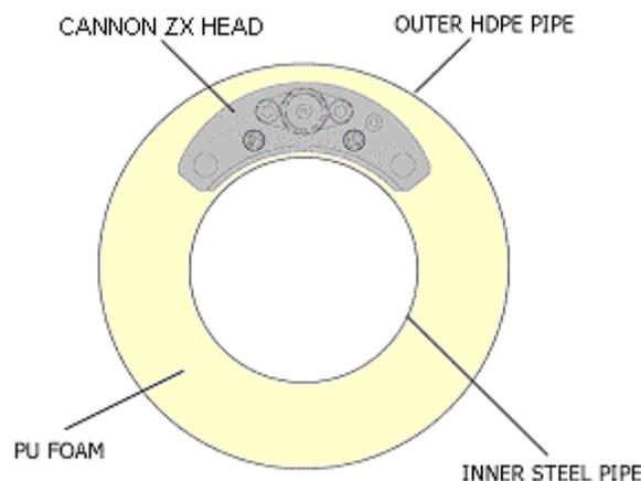
Picture 7 – Pipe-in-Pipe Layout: ZX Head is positioned in the filling cavity in working condition
