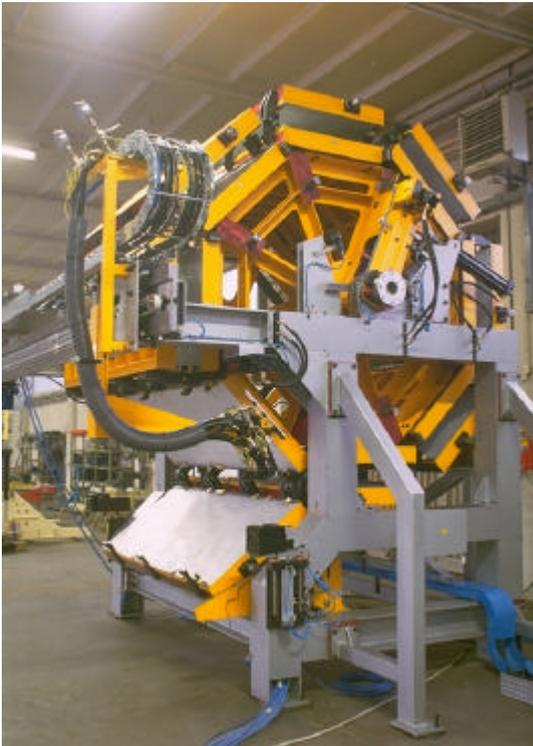
*Picture 3 - DRUM-6, a Cannon Crios development, is a compact production tool for refrigerator doors and small panels.*
