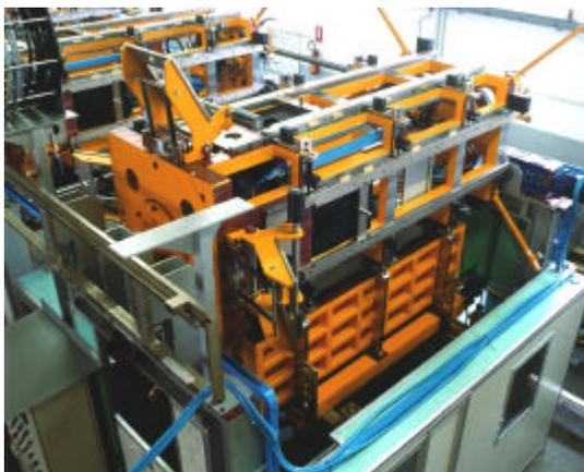
Picture 7 - ROTOPLUG-4 is now currently used in production of large commercial refrigerators.
