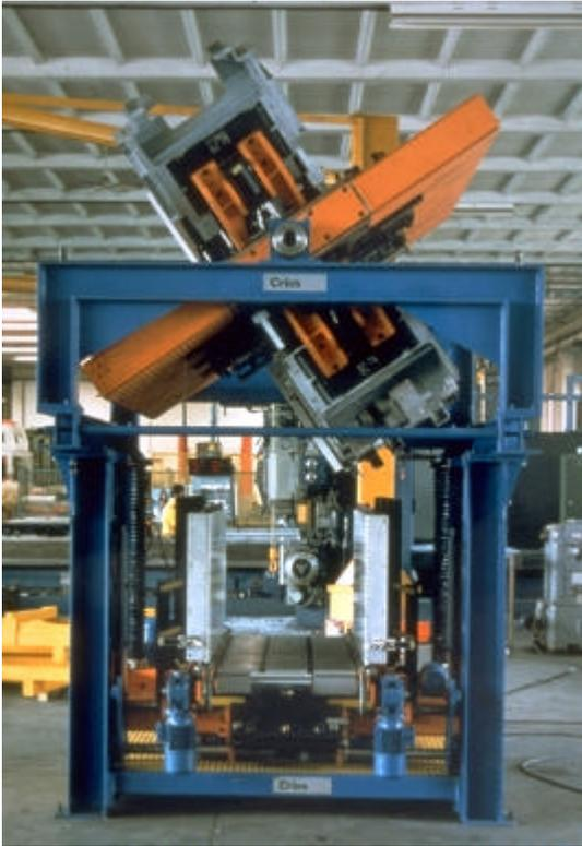
*Picture 1 - Patented by Cannon in the early 1980's the ROTOPLUG fixture guarantees zero-time-plug-change with numerous advantages in production and in economics.*
