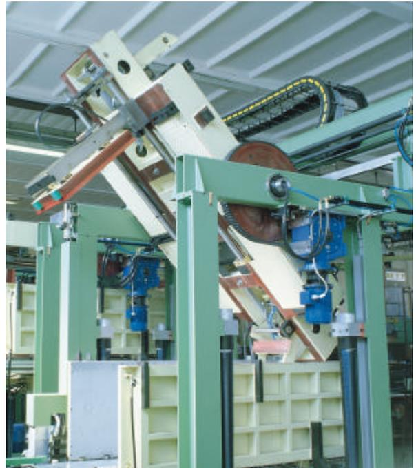
*Picture 4 - This new version of ROTOPLUG - rotating on the longer fixture's side - is very adapt to the longer and heavier plugs.*
