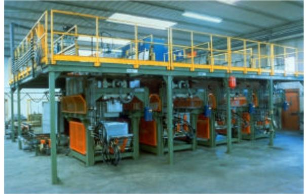
*Picture 2 - ROTOPLUG-4, here shown in a configuration of four units, allows four different plugs to be always available for immediate foaming*
