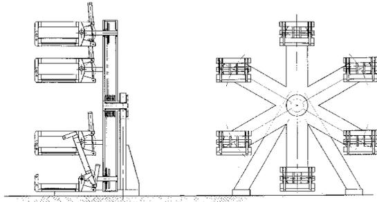
Picture 11. The FlexiDrum rotary polymerization system is a compact solution for the production of automotive seats.
