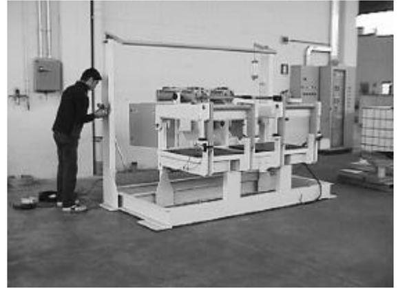
*Picture 9. Each moulding line incorporates an independent station where service operations can be performed without disturbing the production cycle.*
