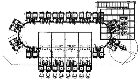
Picture 11. The In-Situ Foaming Carousel provides a row of service positions where time-intensive manual operations can be performed without penalising the efficiency of the moulding line.
