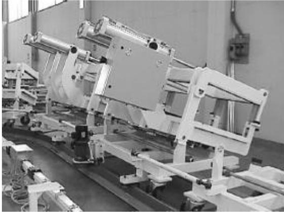
*Picture 8. Mould carrier tilting, which ensures optimal evacuation of air during the filling phase, can be actuated hydraulically or mechanically.*
