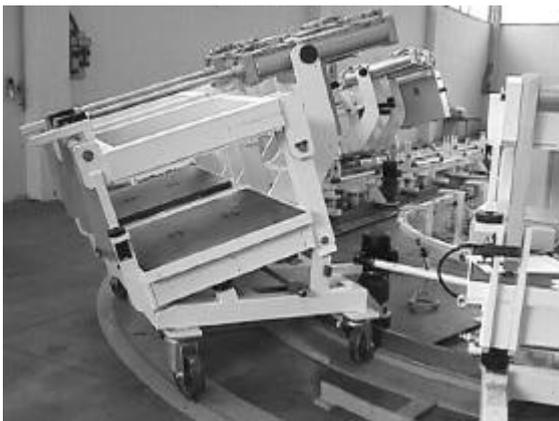
*Picture 7. The flexible foam moulding system incorporates mould carriers with two independent upper and two independent lower platens to compensate for any difference in mould thickness.*
