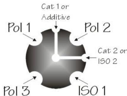
Picture 4. The four main components are fed into the mixing head radially while the two lower-volume streams are fed axially.
