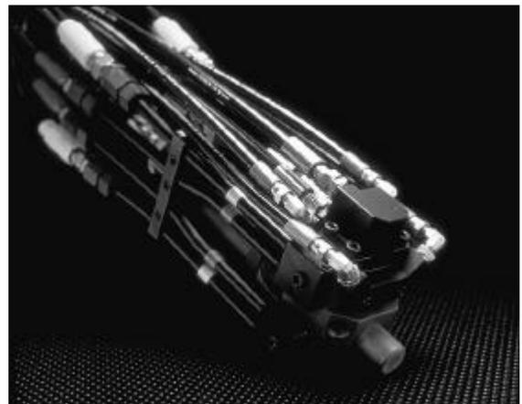
Picture 3. Cannon's new FPL-AX is capable of mixing six components, each with individual recirculation control.
