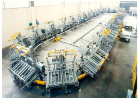
*Picture 10. The idle wheels running along the central guide plate maintain the mould carrier on its path.*
