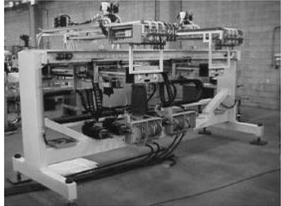
*Picture 6. Cannon's double-arm pour robot is typically designed to carry two mixing heads.*
