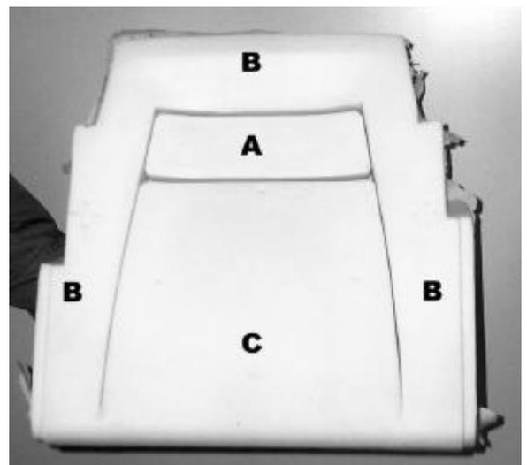
Picture 12. Using natural carbon dioxide for expansion of the foam with Cannon's multi-component mixing head enables a seat with three different hardnesses to be produced.
