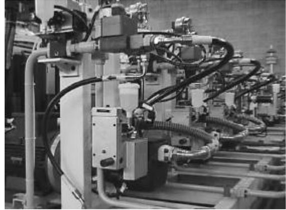
Picture 2. The output control system on Cannon's "A-System" Servo multi-component metering unit operates continuously.
