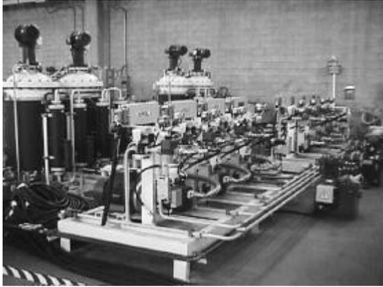
Picture 1. The modular design of the "A-System" Servo includes a set of day tanks, a temperature conditioning system, a metering system and appropriate controls.
